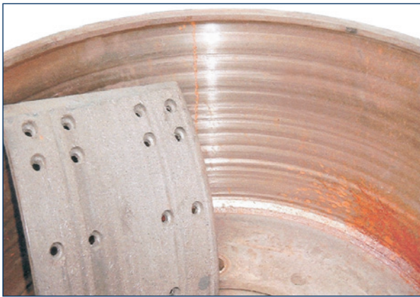
a) Scoring due to coarse dirt
