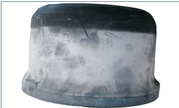
Scorches and temper colours with heat cracks starting to form
