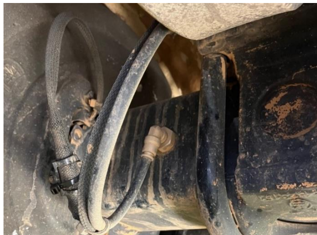
Figure 3: Example of the new exit hole location on an axle
